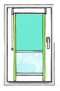
We unstick protecting foil from the guides. We draw the guide on slightly pulled out roller blind and stick it along interior edge of frame of the window/on the joint of glazing bead with frame of the window. We can use spirit level to help.
