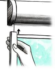
At the end we stick the handle for the chain of roller blinder, so that it is slightly taut.
