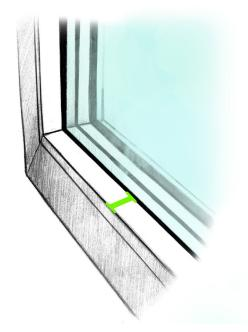
We have to pay attention also to dimension of the width of glazing bead. It must have at least 1 cm(the width marked in figure) for standard clamping.
